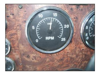
Once engine fluid levels have reached normal operating conditions the Carbon Balance study may begin. The above photograph shows that the engine RPM is locked in place at 1400 r.p.m., which in this case is the approved operating rpm with the mixer drum at full speed. It should be noted that any deviation in r.p.m., temperature, either fluid or exhaust, would cause this unit to be eliminated from the evaluation due to mechanical inconsistencies.
