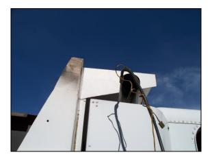
While the emission-sampling probe is in place, and data is being collected, exhaust temperature and pressure are monitored throughout the entirety of the Carbon Balance procedure. This photograph shows the typical location of the exhaust emissions sampling probe.
