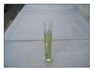
Fuel density and temperature tests are performed for both the baseline and treated segments of the evaluation to determine the energy content of the fuel. A .800 to .910 Precision Hydrometer, columnar flask and Raytek Minitemp are utilized to determine the fuel density for each prescribed segment of the evaluation.
