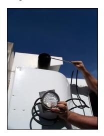
The above photograph shows one method in which exhaust pressure can be monitored during the Carbon Balance test procedure. In this case, exhaust pressure is ascertained through the use of a Magnahelic gauge. This type of stringent regime further documents the inherent accuracy of the Carbon Balance test.
